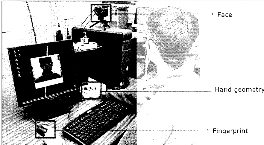
Figure 2.2. A multimodal interface to acquire face, fingerprint and hand geometry images of a person. A well designed interface can enhance user convenience and ensure that multiple sources of evidence are reliably acquired. In this example, integrating the hand and fingerprint input devices into a single unit may be beneficial as it would reduce the burden on the individual to explicitly interact with two spatially separated devices.
